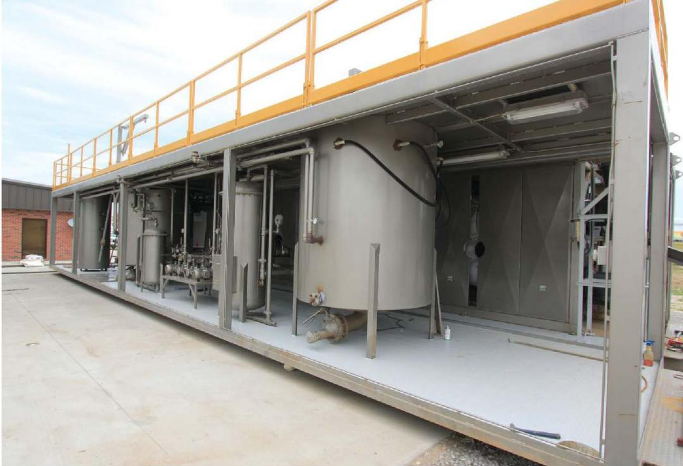
Above is a look at the inside of a typical indirect fire thermal desorption unit with vapor recover unit from Vulcan.
